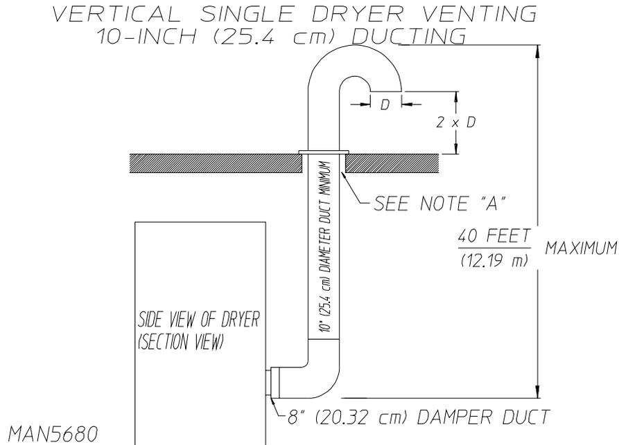
NOTE A: OPENING MUST BE 2-INCHES (5.08 cm) LARGER THAN THE DUCT (ALL THE WAY AROUND).
