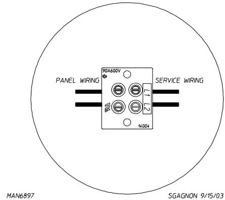
A ground lug is provided in the rear electrical box to connect your service ground.
