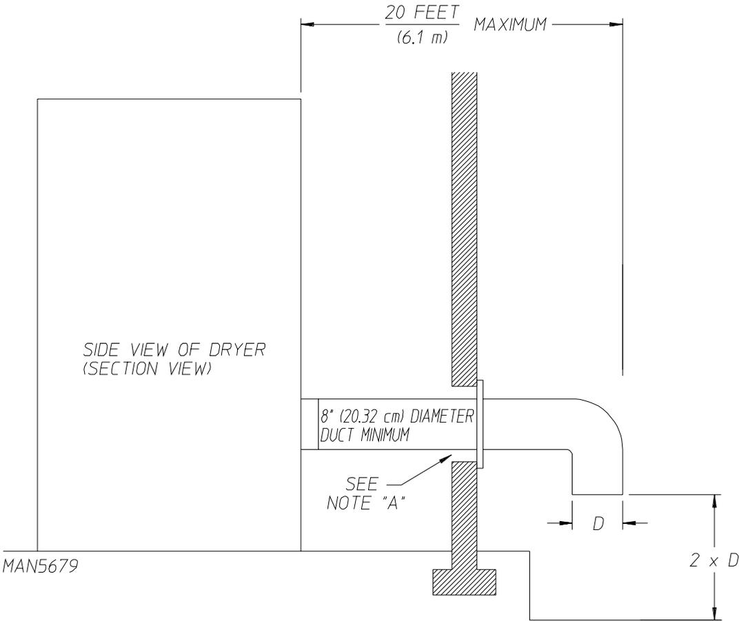
NOTE A: OPENING MUST BE 2-INCHES (5.08 cm) LARGER THAN THE DUCT (ALL THE WAY AROUND). THE DUCT MUST BE CENTERED WITHIN THIS OPENING.
