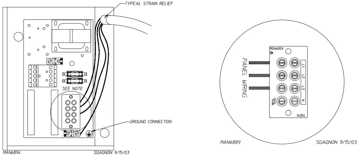
The neutral will only be used on 4-wire service. This is typical for 380-416V, 50 Hz.
